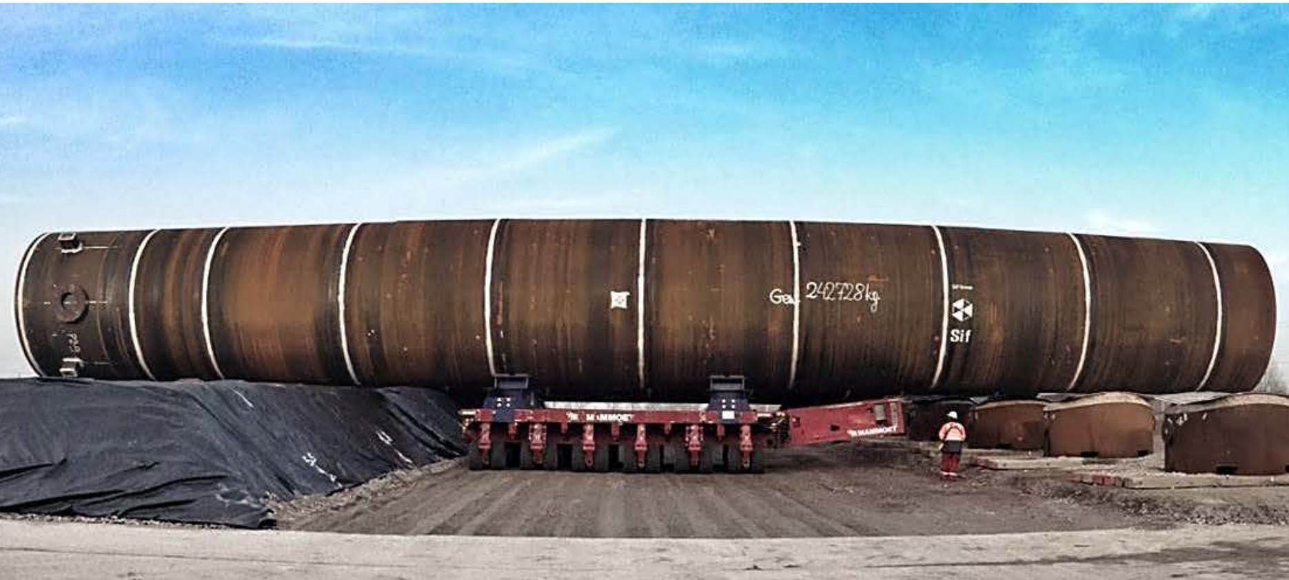
Sif to produce mono pile foundations for wind turbines at Maasvlakte 2
