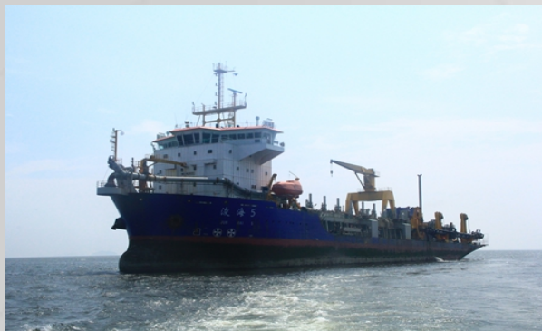
TSHD "Junhai 5" from Guangzhou Dredging Co., capacity of 10,000 m 3
