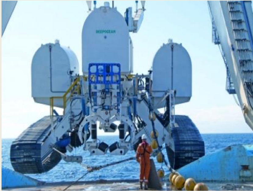
Chain cutter trencher 'T3200' (Deep Ocean Group)
