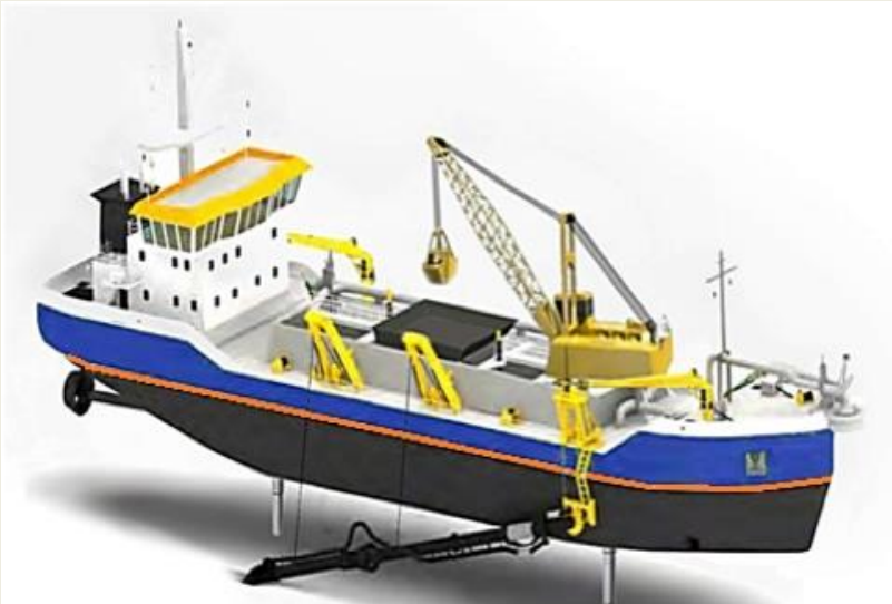
Trailer hopper suction dredger '1000 M3' (Hydromec Maritime Solutions 2015)
