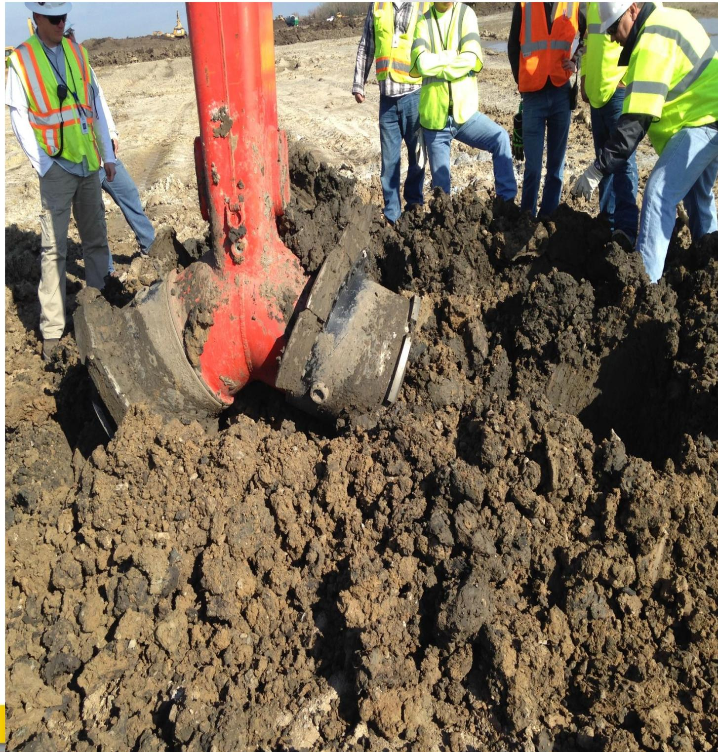
Testing consistency of soil subject to treatment. PMX operated without binder. Note high clay & silt content evidenced by soil “smear”
