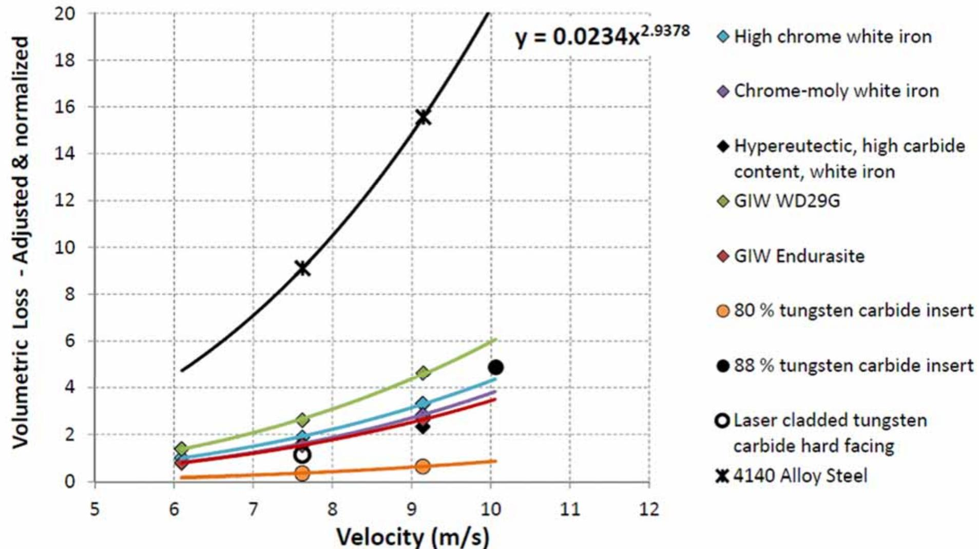
$$W_{VL} = \frac{1}{\left( \underline{C_{VL}} \times \left( \frac{TPH_{ref}}{\underline{TPH_a}} \right) \times \left( \frac{\underline{V_{Iref}}}{V_{Ia}} \right)^{\underline{ExpV}} \times \underline{W_{rel}} \right)}$$
