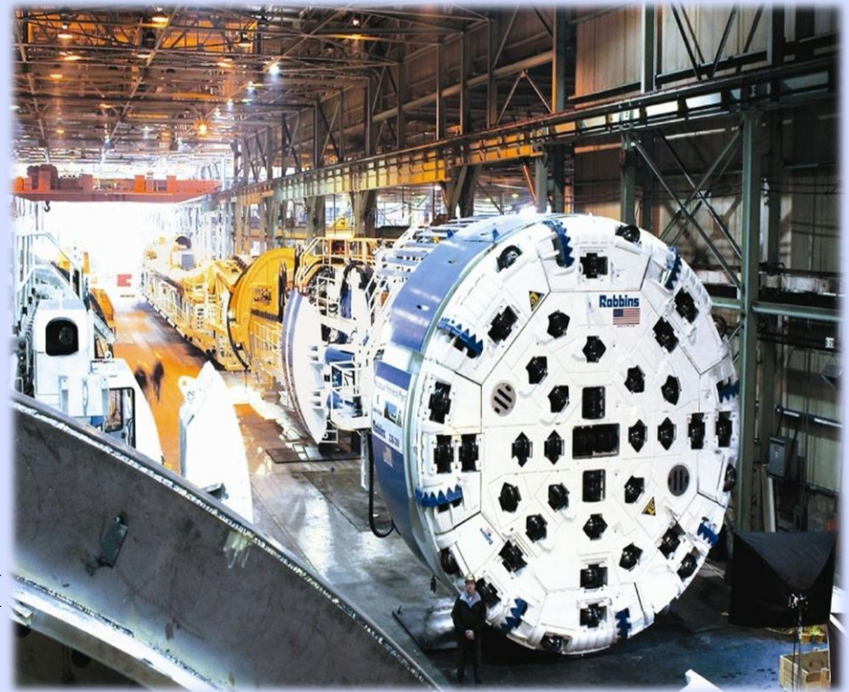
Tunnel Boring Machine
