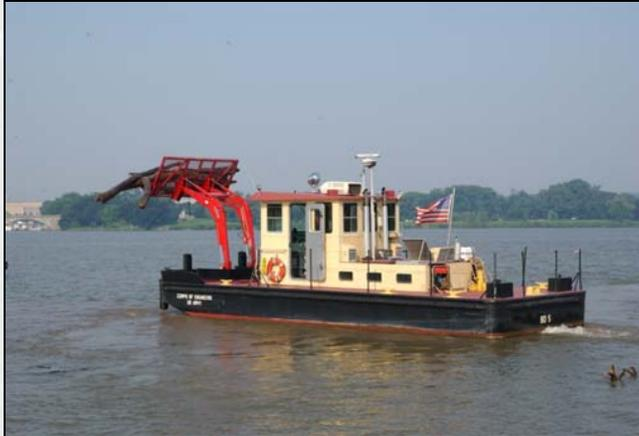
The *BD-5*, a drift collection vessel based in Washington, D.C.
