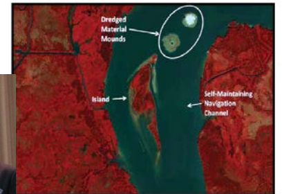
Figure 1. December 2011 aerial infrared photograph of the Atchafalaya River island after multiple years of systematic monitoring of dredged material. The island's formation has reduced the overall cross-sectional area of the river, decreasing river flow through the navigation channel to the east sufficient to reduce channel and maintenance dredging requirements.
