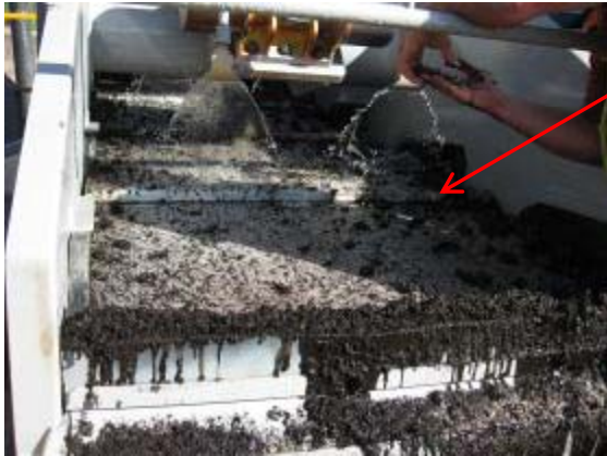
Lead Shot Recovery From Hydro-cyclone
