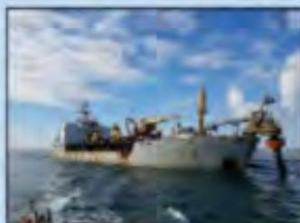
Dutra Group dredge Stuyvesant anchored with the pump-ashore pipe attached
