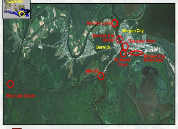
Type of Equipment: Cutterhead Schedule: Jul - Oct 2019 Depth: 12 ft to 16 ft Width: Various Quantity: 1.2M cy Placement Areas: Open Water Sand Pits (Berwick Harbor) Last Dredged: 2018
