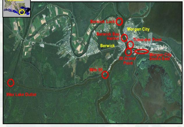
Type of Equipment: Cutterhead Schedule: Jun - Oct 2017 Depth: 12 ft to 16 ft Width: Various Quantity: 1.2M cy Placement Areas: Open Water Sand Pits (Berwick Harbor) Last Dredged: 2016
