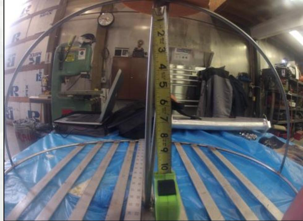
Prototype deployable deposition meter, via Curtis Roegner-NOAA. These are designed to go “over the side” and be retrieved like crab traps.
