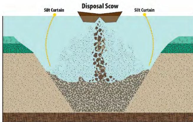
4. Unsuitable Material Placement
