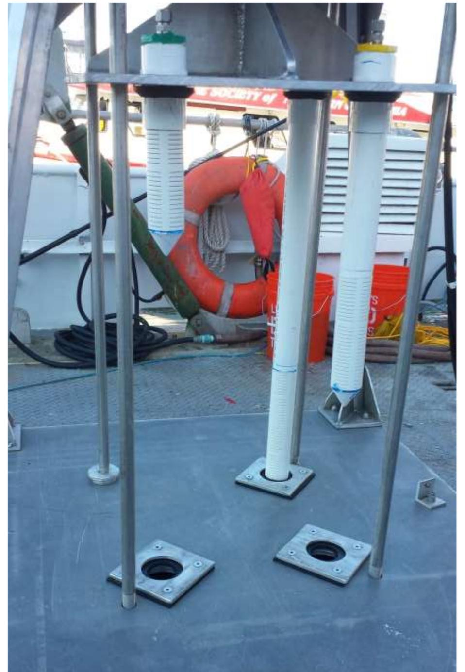
Each pore water interval, plus surface water, has dedicated PVC screen and tygon tubing
