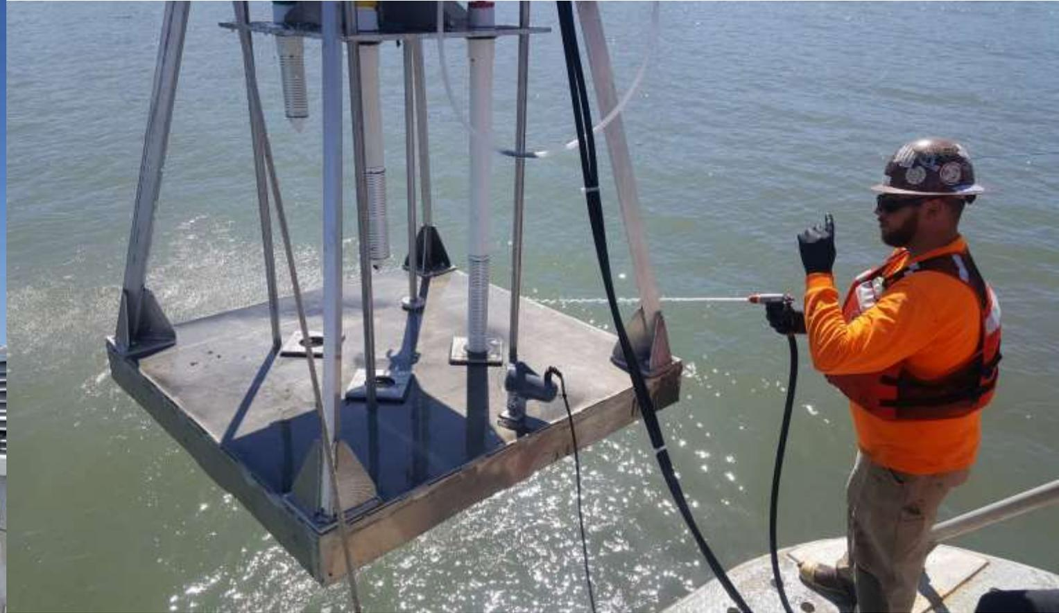
Assembling screens to collect samples from three depth intervals;
