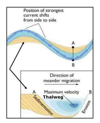
Thalweg: the line of lowest bed elevation or maximum flow depth in a watercourse.
