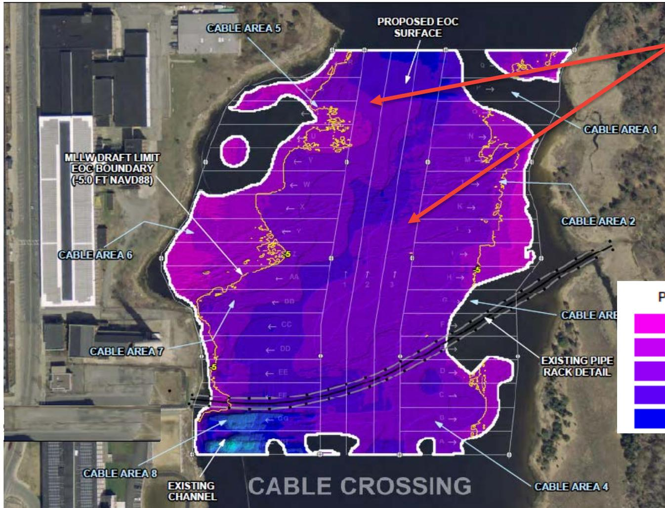
Center lanes will be dredged first to allow vessels to move with moving contaminated sediment within dredge area. Propeller will be strictly controlled.
