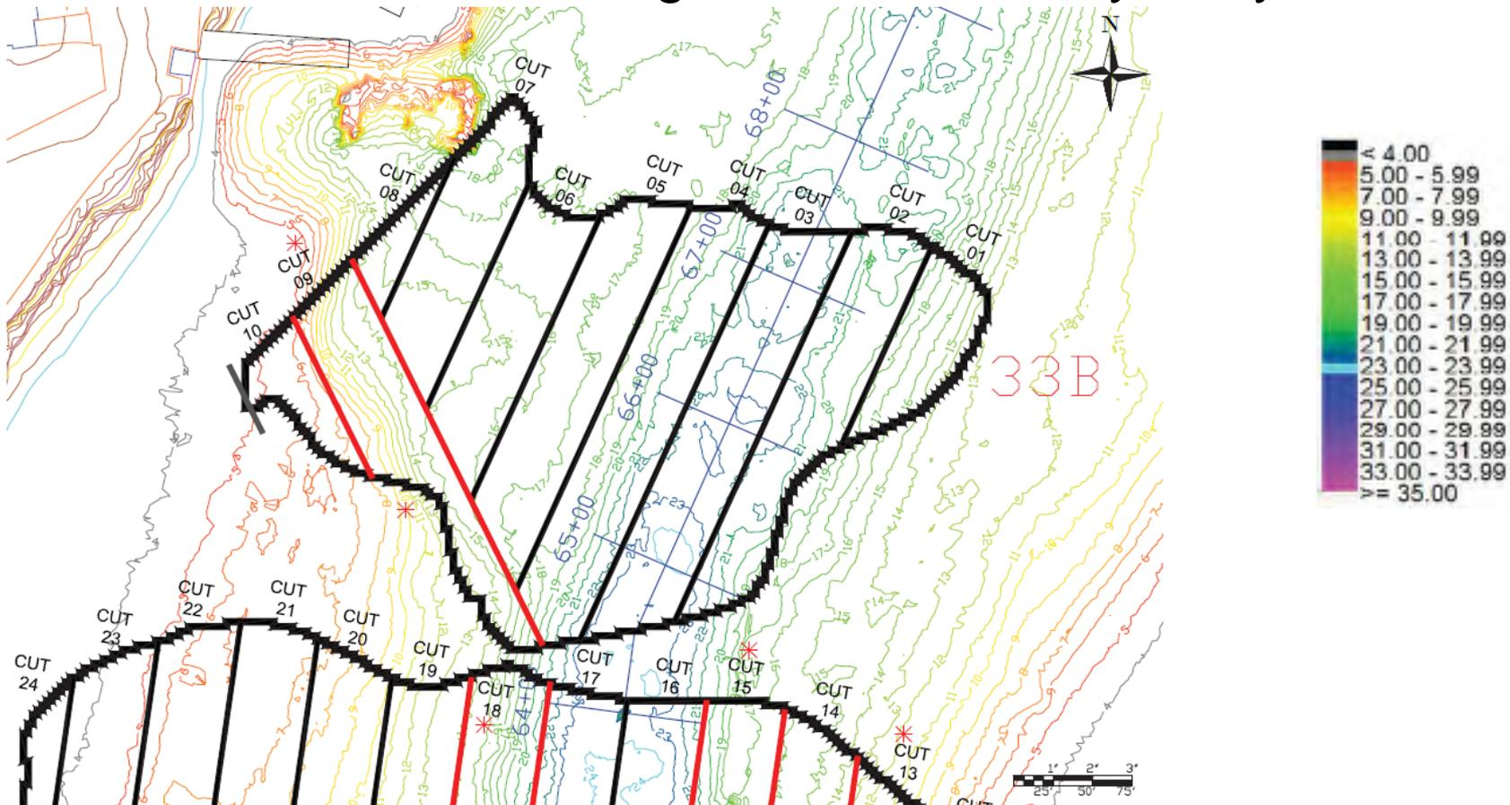
Each dredge area will be setup with 50' cut lanes that run parallel to the natural slope.
