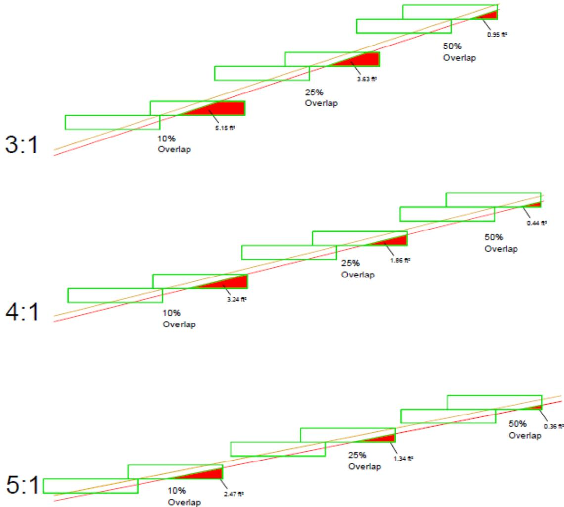
Balancing over-dredge with production rate
