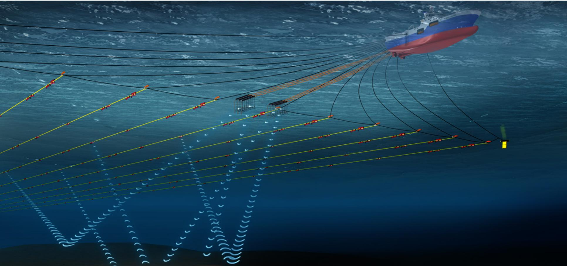
Seabed geophysics may use active or passive methods. Acoustic signal reflection, refraction, electro-magnetic resistivity and passive magnetometers make up the most common methods.
