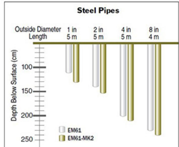
Geomatrix EM-61S: Detection depth for Steel Pipe
