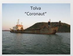
2,500 m<sup>3</sup> Hopper capacity Loading capacity 3,500 Ton
