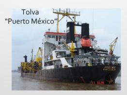
Hopper capacity 4,000 m<sup>3</sup> Loading capacity 7,280 Ton
