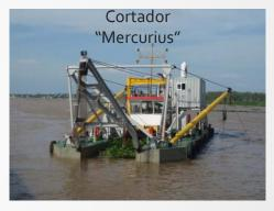
700 mm Diameter of the suction tube 700 mm Diameter of the unloading tube Total power installed 3843 Kw
